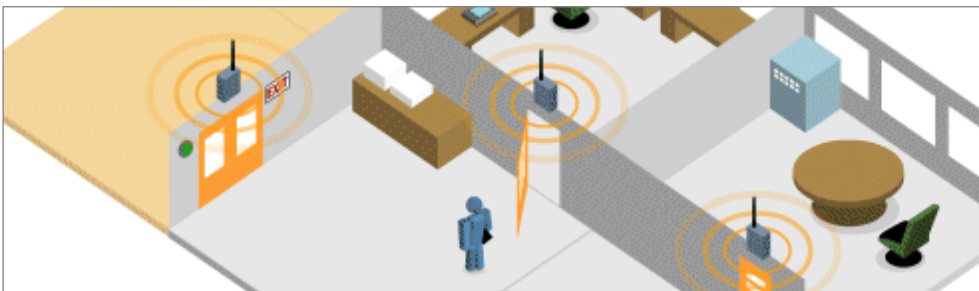
RFID tag and reader helps pinpoint individuals within the building.
